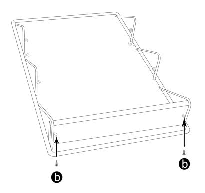
Screw the wooden shelves into the screw slots on the wire.
